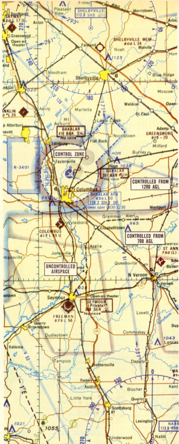
Figure 1. A portion of the Cincinnati Sectional aeronautical chart, illustrating the method of depicting a control zone, controlled airspace having a floor of 700 feet above the earth's surface, controlled airspace having a floor of 1,200 feet above the surface, and uncontrolled airspace. The limits of controlled airspace are color-coded in magenta and blue. The dark edge of the vignette indicates the limit of controlled airspace, and the vanishing edge the direction of controlled airspace
